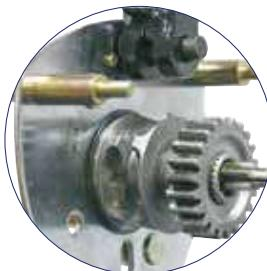
Load sheave with closed ballbearing
